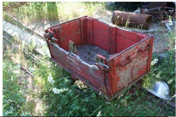
**Left: Rails Bridging Sherlock Creek About Five Feet Above Bed. Note the Stone Dressed Stream Bank. Right: Ore Cart on the Rails to Move Rock from the Mine to the Sluice Box Across Sherlock Creek.**
